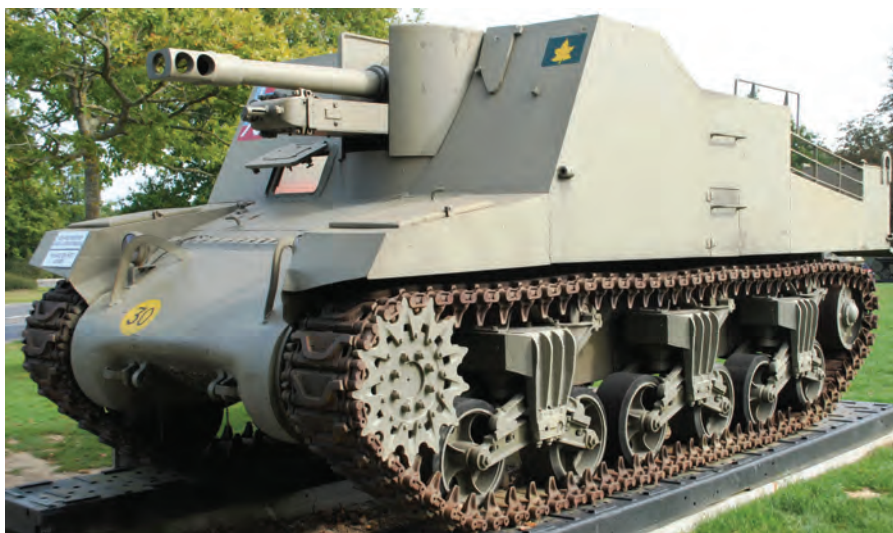
A Canadian Tank Destroyer built on a Sherman chassis and fitted with a 25 pounder gun.
