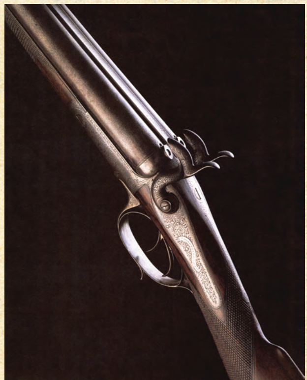
An Edward Harrison pin-fire 12-bore, No. 5,883, with automatic half-cocking mechanism, the subject of his patent No. 271 of 1 February 1864. (E. Rosner collection).
